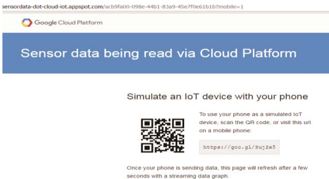
Figure A.2. First page of Ice breaker Demo – practical example of interaction with Google Cloud Platform through mobile device. Offered QR code scan or to type direct hyperlink on a device
