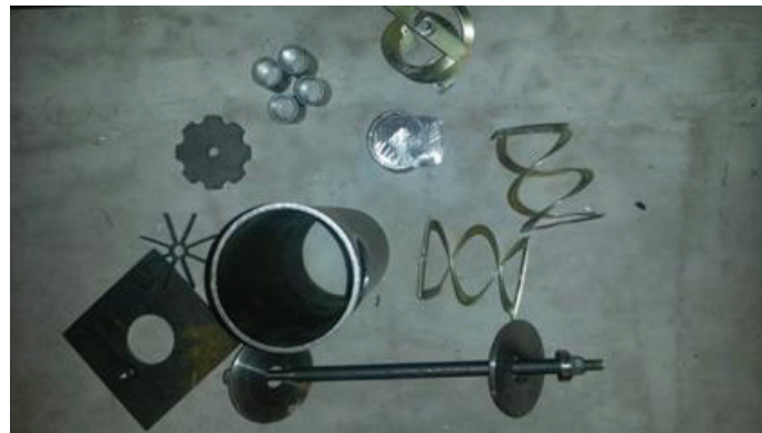
Figure 2 – Fertilizer distributor in unassembled form
