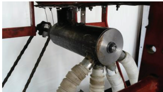
Figure 4 – The seed distributor fixed under the bunker
