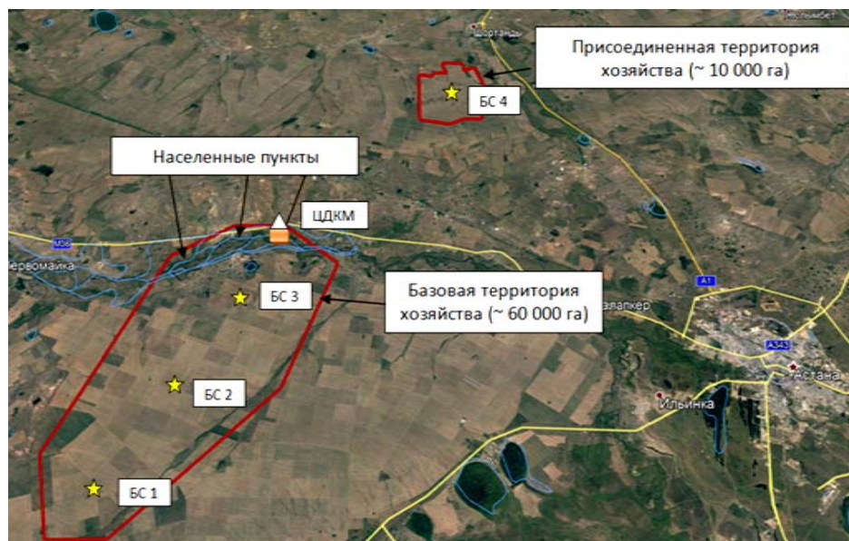
Figure 6 – Layout of BS of differential correction and the CDCM on the territory of the Agro firm
