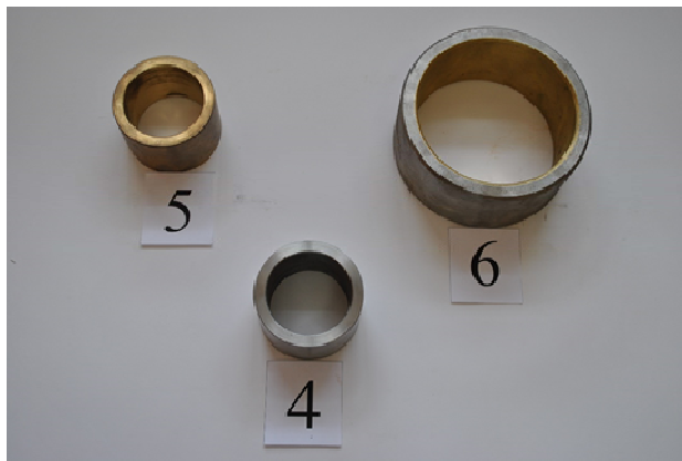
Figure 3 – Construction of the bushings
